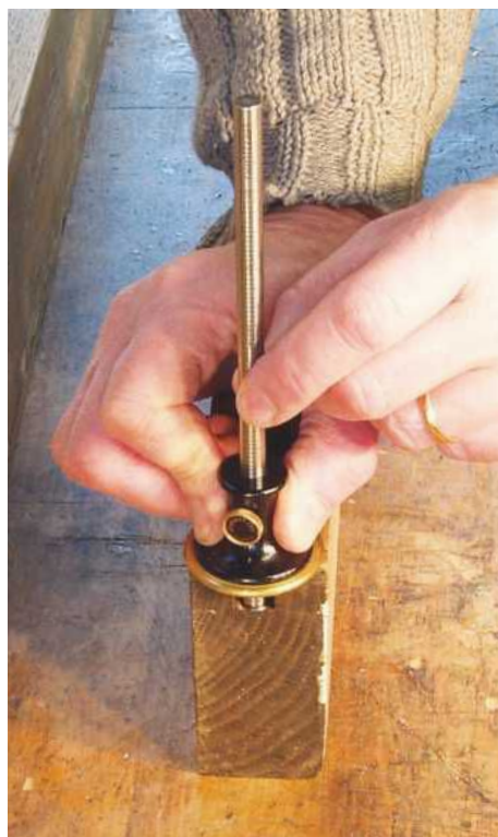
▲ Pic.10 Using the wheel gauge as a depth gauge
